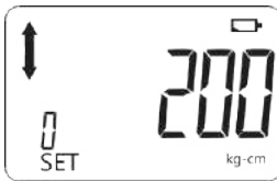
Battery voltage under 2.6V
